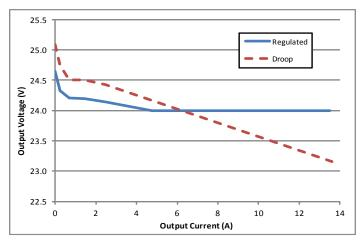
Figure 6: Typical output voltage vs. output current for regulated and droop version outputs.
