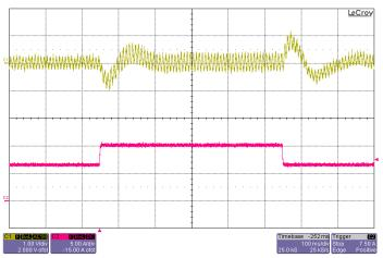
Figure 8: Output voltage response to step-change in load current with  $200\mu$ F hold-up capacitor (50%-75%-50% of Iout(max), 115Vrms, 60Hz) Top: Vout (1V/div), Bottom: Iout (5A/div), Timebase: (100ms/div).
