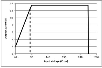
Figure 12: Maximum output current vs. input voltage, output turn-on threshold is 85Vrms.
