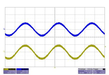
**Figure 3**: Typical Input Voltage and Current waveforms at full load current (115Vrms, 60Hz) Top: Vin (200V/div), Bottom: Iin (5A/div), Timebase: (5ms/div).
