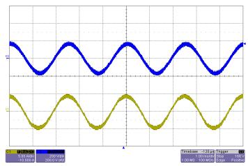
Figure 4: Typical Input Voltage and Current waveforms at full load current (115Vrms, 400Hz). Top: Vin (200V/div), Bottom: Iin (5A/div), Timebase: (1ms/div).
