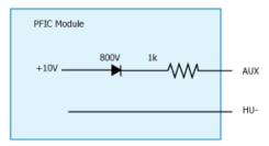
The purpose of the AUX power supply is to provide a low level of power to primary control circuitry, referenced to HU-.
