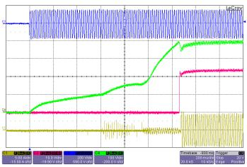
**Figure 9:** Typical startup waveform with 200μF hold-up capacitor (115Vrms, 60Hz) Ch1: Iin (5A/div), Ch2: Vout (10V/div), Ch3: Vin (200V/div), Ch4: Hold-up capacitor voltage (100V/div), Timebase: (200ms/div).
