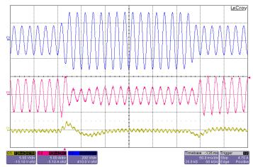
**Figure 10:** Input voltage transient response with 200μF hold-up capacitor at full load current (115Vrms-230Vrms-115Vrms, 60Hz), Top: Vin (200V/div), Mid: Iin (5A/div), Bottom: Vout (5V/div), Timebase: (50ms/div).
