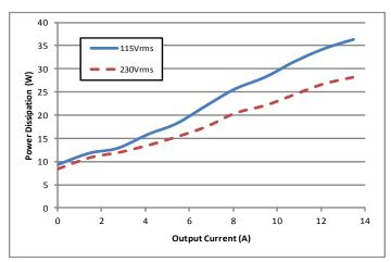
Figure 2: Power dissipation at nominal output voltage vs. load current for 115Vrms and 230Vrms (60Hz) input voltage at Tb = 25 °C.
