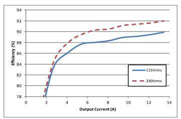
Figure 1: Efficiency at nominal output voltage vs. load current for 115Vrms and 230Vrms (60Hz) input voltage at Tb = 25 °C.
